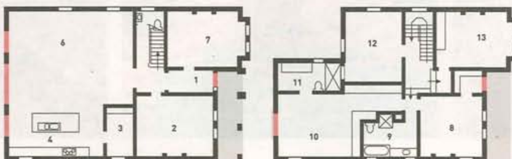
GROUND FLOOR 1 Entry 2 Loungeroom 3 Laundry 4 Kitchen 5 Garage 6 Dining/Living 7 Formal dining room FIRST FLOOR 8 Bedroom 9 Bathroom 10 Main bedroom 11 Ensuite 12 Bedroom 13 Bedroom
